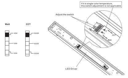
Adjusting the switch, and making the switch fix on the needed Watt and CCT.
