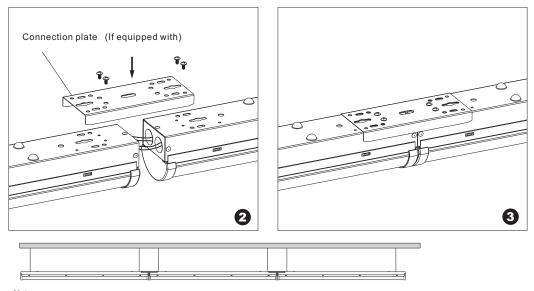
Note: For safety standard, please do not connect more than 4pcs 4ft LED lamp in a row; do not connect more than 3 pcs 8ft LED lamp in a row.
